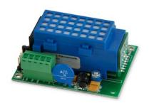
Infrared gas sensor using dual beam technology, with measurement and reference channel, for monitoring room air and process control applications. Integrated  $\mu$ -controller-evaluation electronics for drift and temperature compensation, and standardized analogue and digital interfaces.
