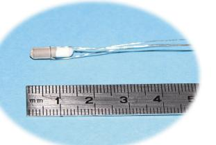
Unlike conventional zirconia sensors, known as "air reference" sensors, MicroPoas<sup>1</sup> obtains its own reference, from a metal and its oxyde both placed and sealed inside a zirconia sheath.
