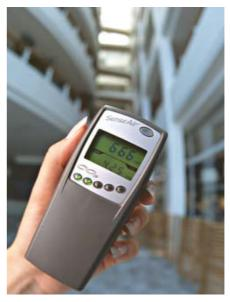
The outer dimensions (125x52x32 mm) make SenseAir® a unique portable gas monitor.
